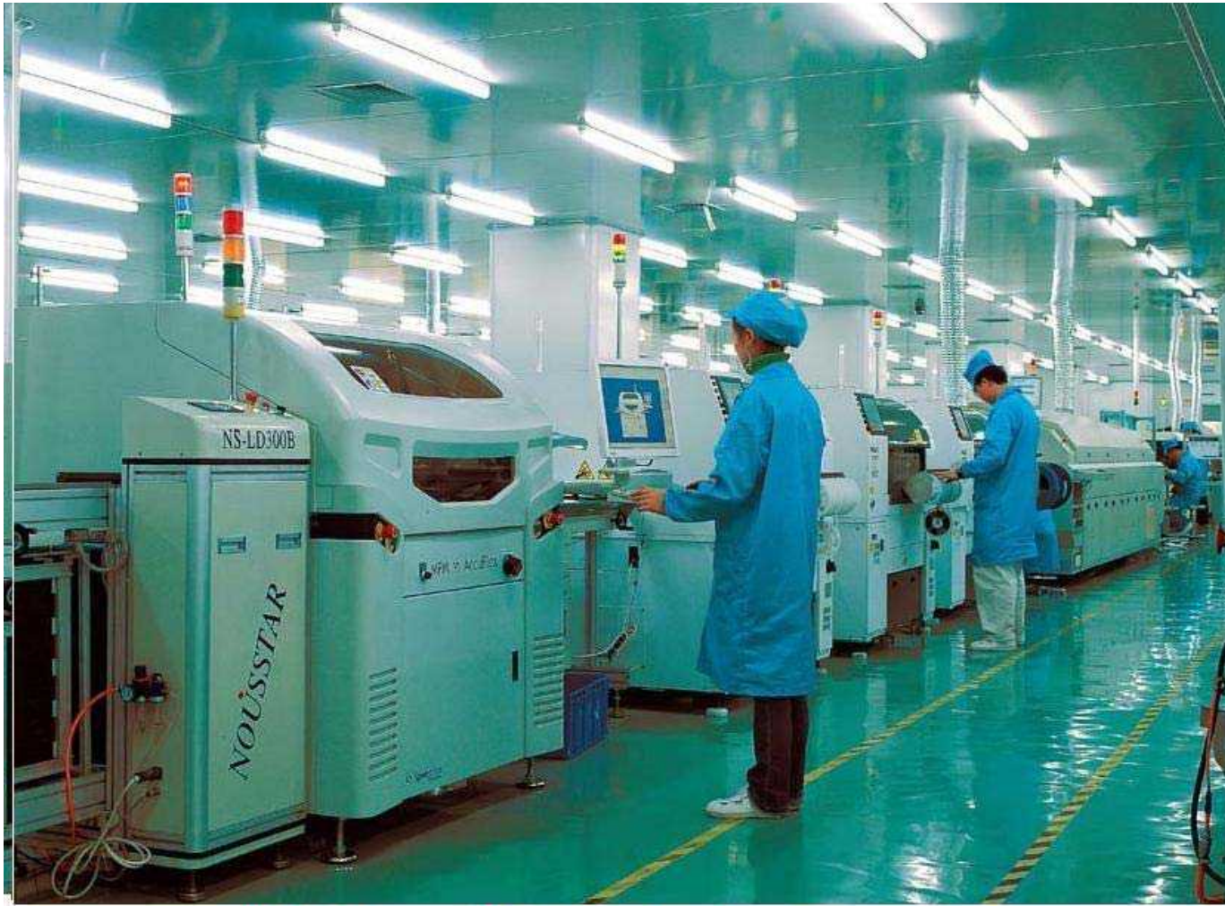
High-Speed SMT Production Line
