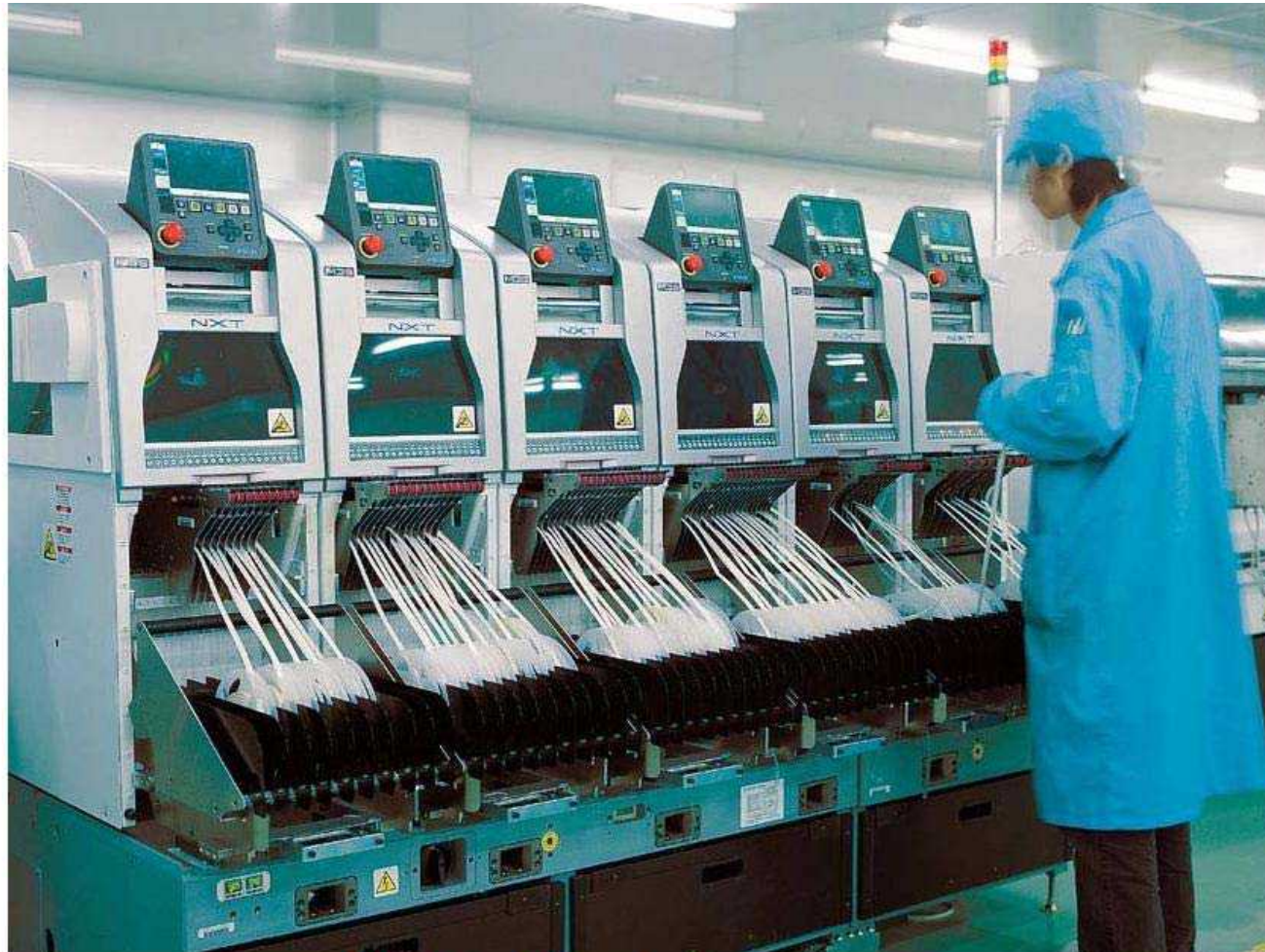
Modular Mounter Room
