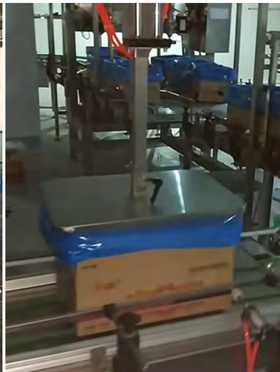
Blowing air to extend inserted bags in cartons
