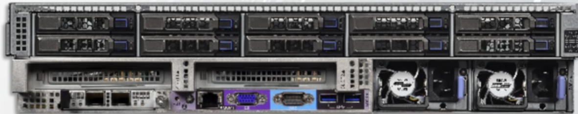
Specially configured model 1: with 10x2.5" hard disk
