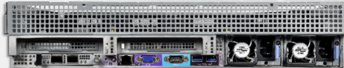
Specially configured model 2: with 4xGPU cards
