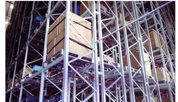
Automatic Storage and Retrieval System
