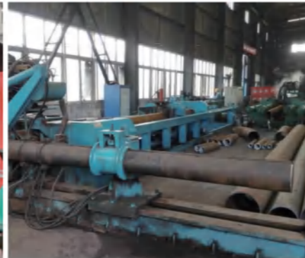
Double-Layer FBE Coating Line
