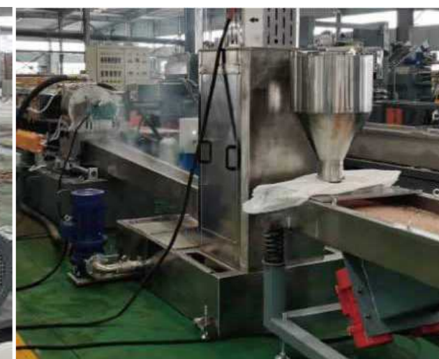
水环模面热切 Hot cutting of water ring mold surface
