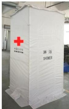
**Material:** The main material is 2 × 2 white silver-coated Oxford cloth, and the frame is made of white plastic-sprayed square 30 × 1.2 welded steel tube and square 25 × 1.2 welded steel tube. The tent is equipped with a floor cloth, a 20L solar camping shower bag, and the tent roof is equipped with a fastening belt to fix the shower bag. The roof is provided with a water inlet and a curtain cloth to prevent water leakage.
