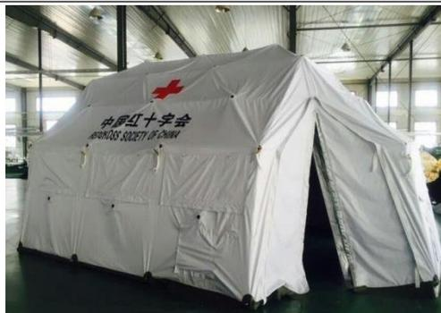
Main material: Fabric: 2×2 silver-coated camouflage waterproof Oxford cloth; Inner layer: 1X1 white waterproof Oxford cloth; ground sheet: 400g/m<sup>2</sup> grass green double-sided plastic coated cloth, frame: medium 16X0.8mm aluminum alloy tube, medium 20×1.5mm aluminum alloy tube, PAI 66, etc.
