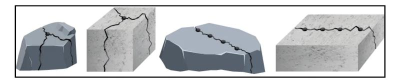
• **Breaking Up Technique:** Boreholes are drilled in offset rows to achieve the smallest fragments. More boreholes result in smaller fragments, with cracking occurring in a criss-cross pattern.
