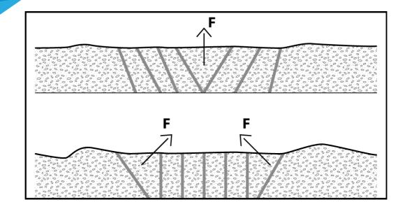
• Rock extraction / rock demolition: There are various techniques for rock extraction or rock demolition. The drilling schedule is selected according to the shape and constitution of the rock or adapted to local regulations. The principle always remains the same. First, try to create a free side, that is, a straight edge. From this edge the extraction can then be continued for as far as is required.
