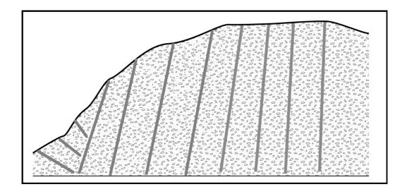
• Excavation Technique: In rock excavation, boreholes are drilled and filled in rows, positioned 5-10 inches [10-15 cm] below the desired ground level. The substrate is broken and loosened, facilitating removal by excavator or, partially, by hand. Optimal effectiveness is achieved when boreholes are somewhat obliquely drilled, allowing a portion of the force to exert upward.
