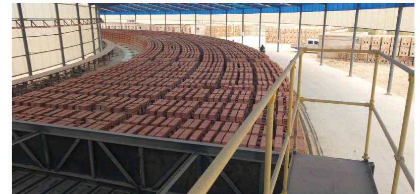
Project: Aksu Dingsheng New Building Materials Co., Ltd Location: Aksu, Xinjiang Kiln Section: 12.98m Kiln Capacity: 400,000-500,000 bricks /day Materials: shale, coal gangue, construction waste
