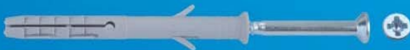
Nylon Frame Anchor Model: FA10100-FA10160 Sleeve: Nylon 6. Screw: Blue/Yellow Zinc Plated.
