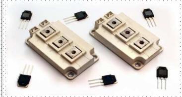
Infineon's IGBT product portfolio provides a broad variety of different devices for a wide range of applications in the fields of automotive, traction, energy transmission, industrial, and consumer systems. These solutions offer very low power losses in the forward and blocking state, only require low drive power, and have a high efficiency.
