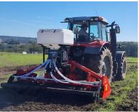
The Seeding Fertilizing Machine is combined with 8 Rows and 150L Pneumatic Seeder, Radar Sensor, Spreading or Drilling Equipment. it's a simple one and it's very suitable for grass seed sowing or fertilizing. This allows farmers to utilise the optimal time for sowing and benefit from saving grass seeds or fertilizer volume and labor cost.
