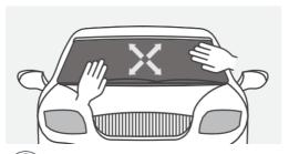
Place the windshield film on the windshield and adjust the position according to the cut size.
