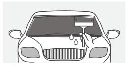
Squeegee from the middle vertical position (No.1) to fix the windshield film, and Squeegee from the top to the outside of the windshield (No.2), to remove the water from the bottom of the windshield. (No.3 to 4)
