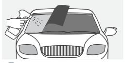
Spray the neutral detergent mixture on the vehicle windshield and the adhesive side of the windshield film without omission.
