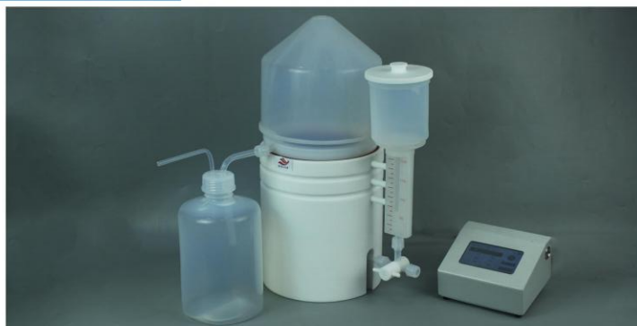
Acid Purification System
