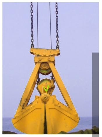
**Structural components:** arms, buckets, and pulley blocks are constructed from high-strength steel conforming to ISO standards.
