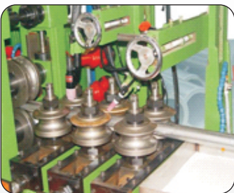
Barrel Corrugation Line
