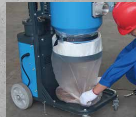
Please tie the bag tightly with the rope and cut it off. pulling the bag down and grabbed by the rope again for next vacuuming.
