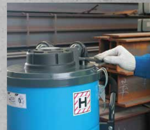
Please turn off the switch and press down the handle, when there is too much dust causes insufficient suction.
