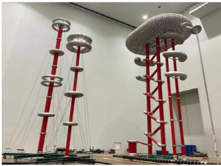
±2000kV DC complete set of experimental equipment
