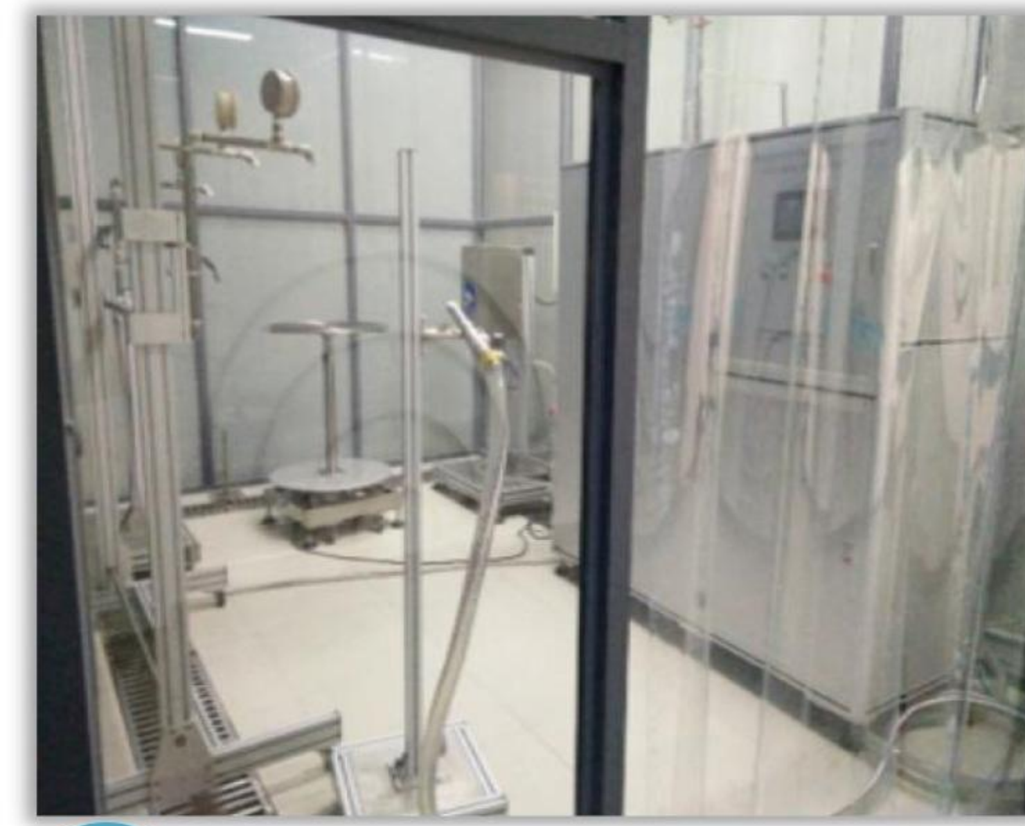
10 IPX3-7UL waterproofing tester
