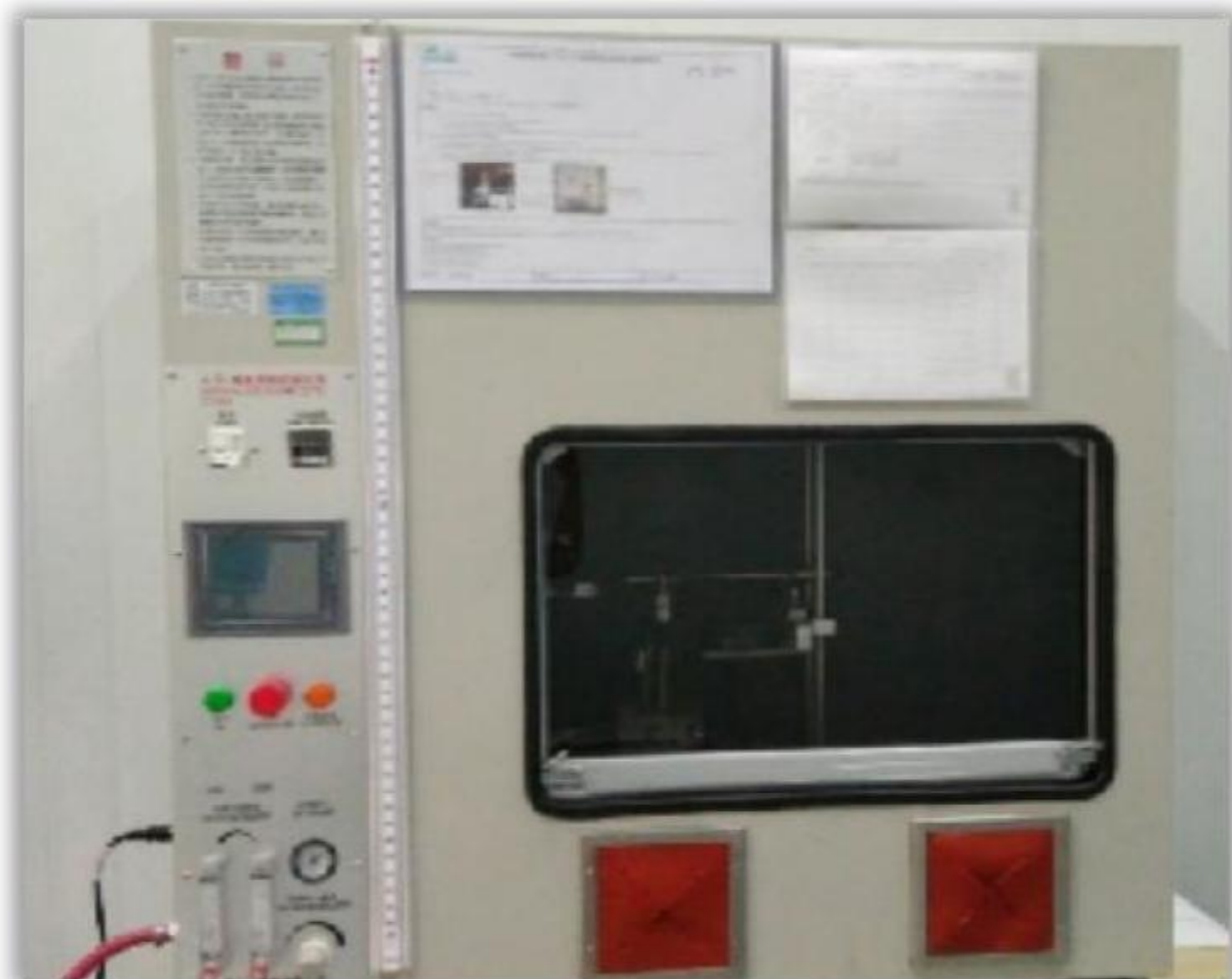
11 Horizontal vertical combustion tester
