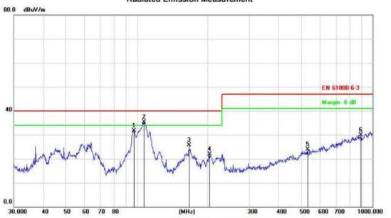
Site LAB Limit: EN 61000-6-3 Polarization: Vertical Temperature:
